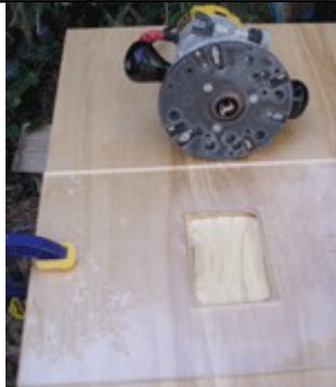
Template clamped to your 3/4" plywood sheet
