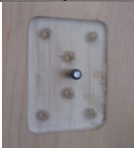
Hole marker plate in plywood. Use a nail to mark the centers to drill.
