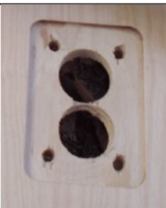
Hole marker plate in plywood. Use a nail to mark the centers to drill.
