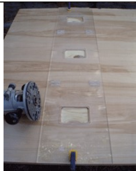
Template clamped to your 3/4" plywood sheet
