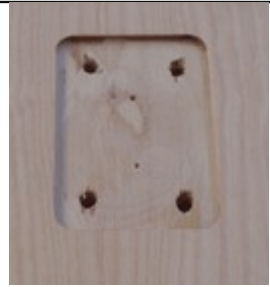
Use a 5/16 drill bit to drill the four corner holes
