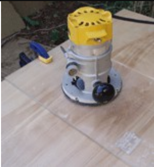
Router placed in the center of the hole in the template.
